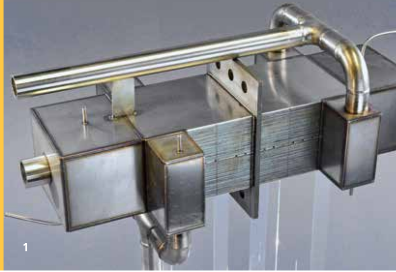
1 Fuel processor for diesel (as part of an APU)
