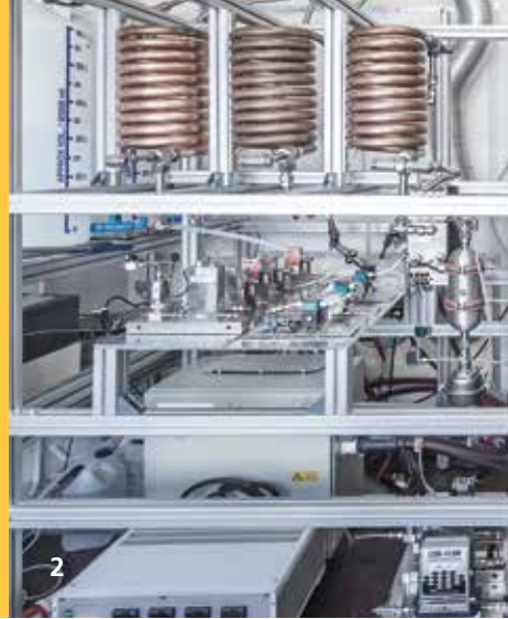
1 Propylene glycol fuel processor 2 Plant for component testing of fuel processor system
